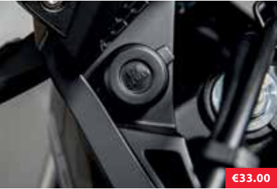
12V SOCKET 08U70-MKP-D80 12V Power Socket allows you to power or charge electrical equipment directly from the bike.
